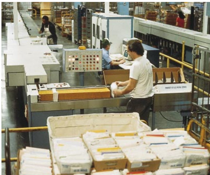
POSTAL-CHARACTER READERS , such as the ones shown here, will be supplemented by devices that can discern handwriting and hard-to-read type on envelopes.
