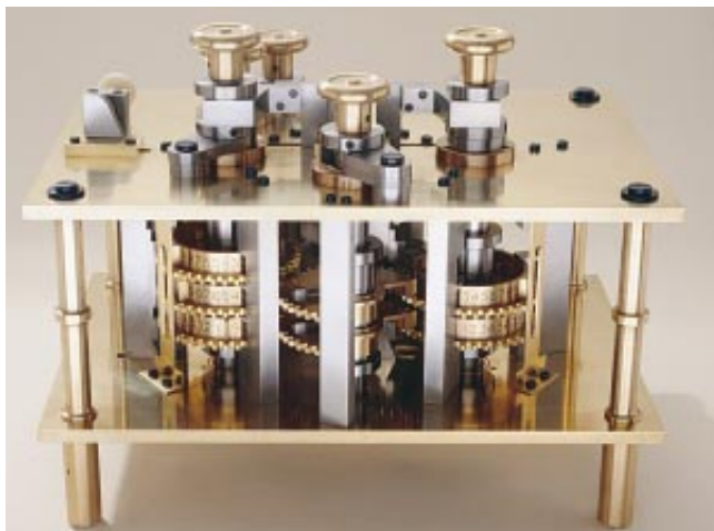
ENGINEERING CHALLENGES were solved in the course of building Difference Engine No. 2. Engineers at the Science Museum constructed a part of the calculating mechanism (left) in 1989
